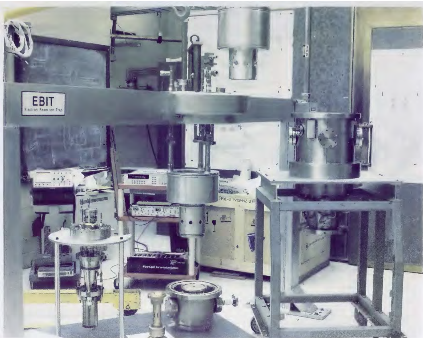
Figure 1. The NIST EBIT, just before final assembly of the 6 major subsections (clockwise from the bottom: electron gun, drift tube assembly, collector, liquid helium insert, liquid nitrogen shield, outer vacuum can).
