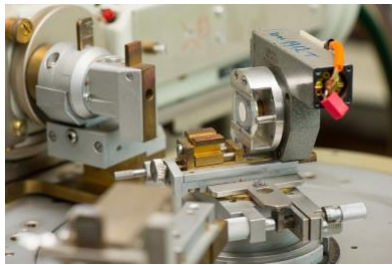
Siemens type X-ray diffractometer with horizontal sample holder and \text{CuK}\alpha 40 kV-40 mA line focused X-ray source
