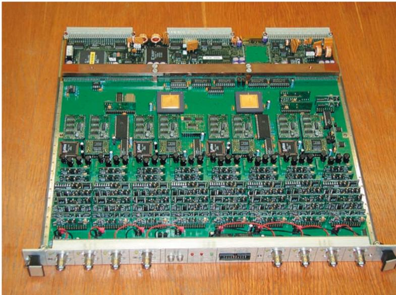
**A unit of the electronic signal processor of the detector system Diamant** shown in the previous picture. It processes the signals of eight CsI(Tl) detectors simultaneously. The information on an impinging particle is extracted from the shape of the electronic signal. The device has been developed in Atomki.
