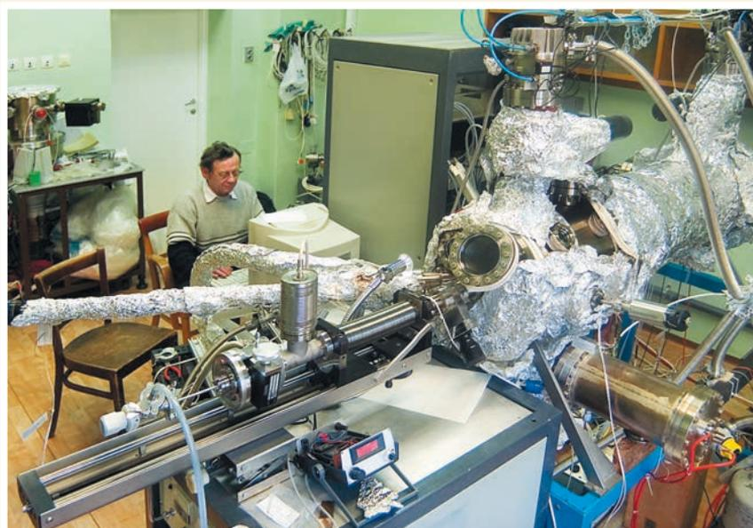
ously. The aluminium foils covering the spectrometer are to improve the effect of the heating wires underneath. The heating helps to produce good vacuum ('ultravacuum') in the spectrometer.
