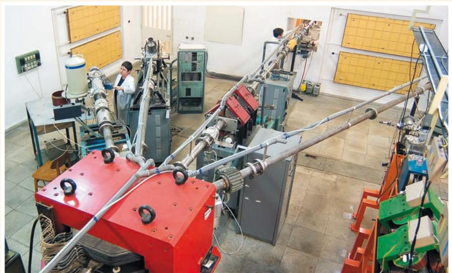
Every channel is equipped specifically, for experiments of a particular type. The picture shows the **experimental channels of the 5-MV Van de Graaff accelerator**. The beam is directed to the desired channel by an electromagnet (painted red in the foreground).
