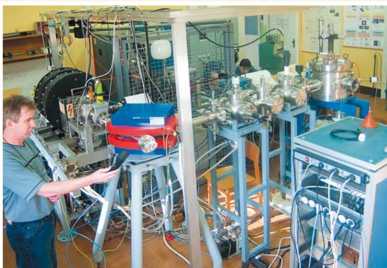
In low-energy electron spectroscopy the energy and angular distribution of electrons is measured. It provides a broadly applicable method for studying the structure of atoms, molecules and solids. In Atomki there are several home-made devices of this type. The **electron spectrometer ESA-21** shown in the picture is unique in that it can provide the energy and angular distribution data of electrons simultane-
