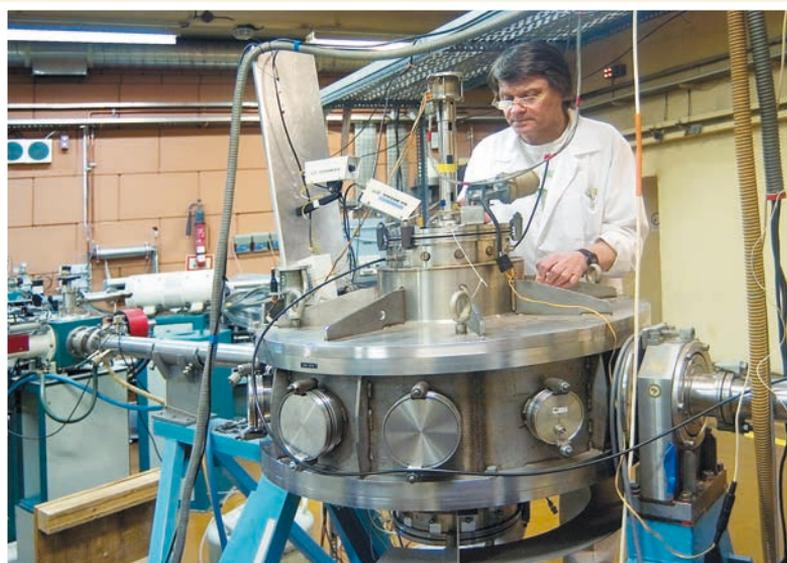
The **vacuum chamber** shown in the picture is installed at one of the beam channels of the cyclotron. In the chamber there are semiconductor detectors, which measure the properties of the particles emerging from the target put in the middle. Some of the reactions studied are replicas of
