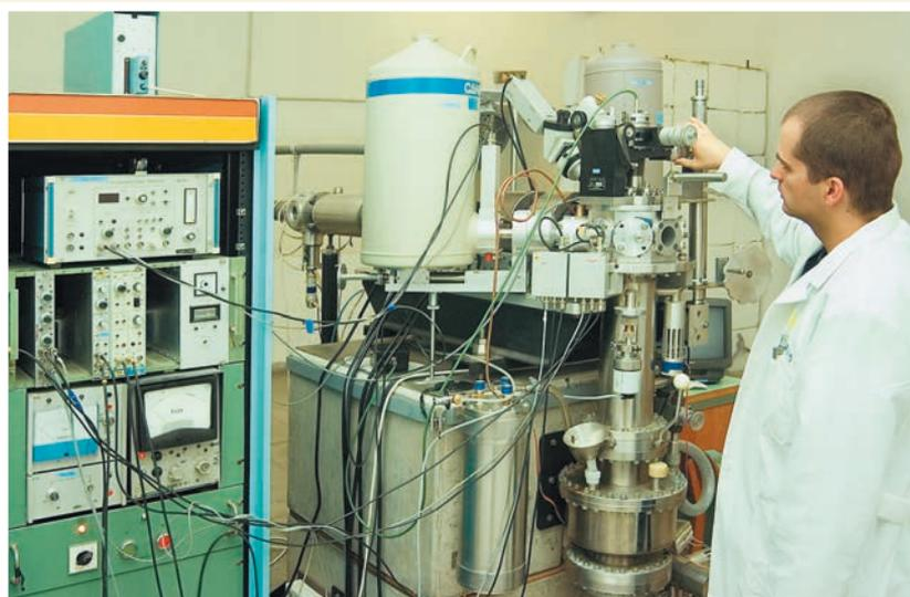
There are several methods to determine the elemental composition of a sample by bombarding it by an ion beam of an accelerator. In some studies the subject of the analysis is the composition of individual small grains of a substance. For such a purpose, the diameter of a usual beam (a few
