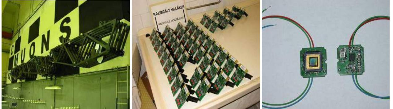
**Figure 21:** Components of the CMS position alignment system: MABs, LEDs, and video sensor left to right.
