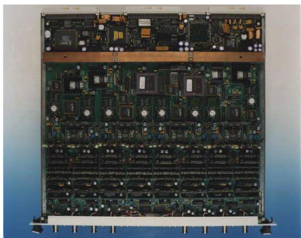
**Figure 14:** VXI module with eight identical channels.
