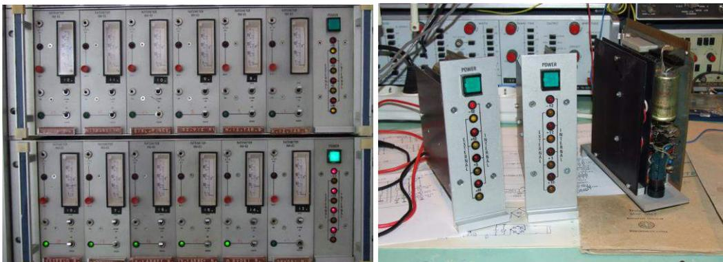
**Figure 9:** Rack of RM-83 rate meters and the maintenance of the power supplies.
