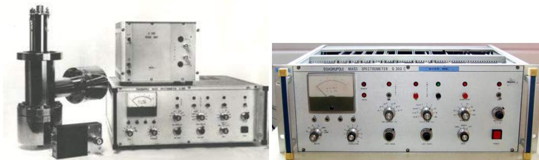
**Figure 8:** The QMS 300 quadrupole mass spectrometer controller and the electronic units and measuring head on left and the Q300C on right. Some parameters are adjustable by computer control in Q300C. Its mass range is 1-300.
