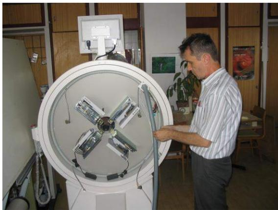
**Figure 37:** The assembly of the miniPET-I small animal PET scanner (J. Molnár).
