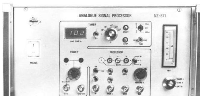
**Figure 7:** NZ-871 Analogue signal processor
