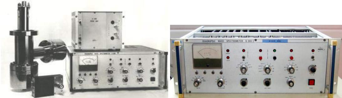
**Figure 8:** The QMS 300 quadrupole mass spectrometer controller and the electronic units and measuring head on left and the Q300C on right. Some parameters are adjustable by computer control in Q300C. Its mass range is 1-300.
