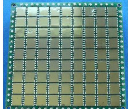
**Figure 51:** SiPM tile of the miniPET-III detector module, manufactured by ST Microelectronics.
