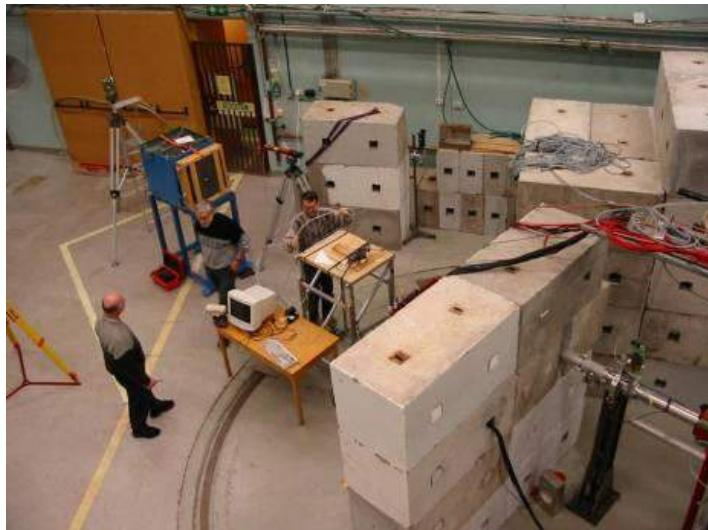
**Figure 23:** PC-104 irradiation setup at TSL, Uppsala. The experiment was carried out by D. Novák, A. Kerek and L-O. Norlin.
