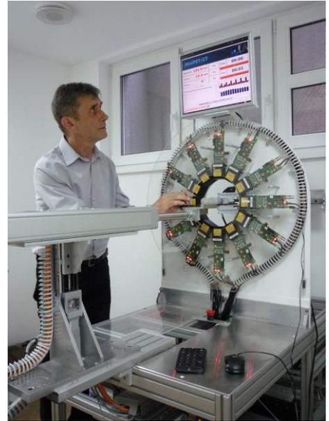
**Figure 44:** Photo of the miniPET-II full ring small animal PET scanner.
