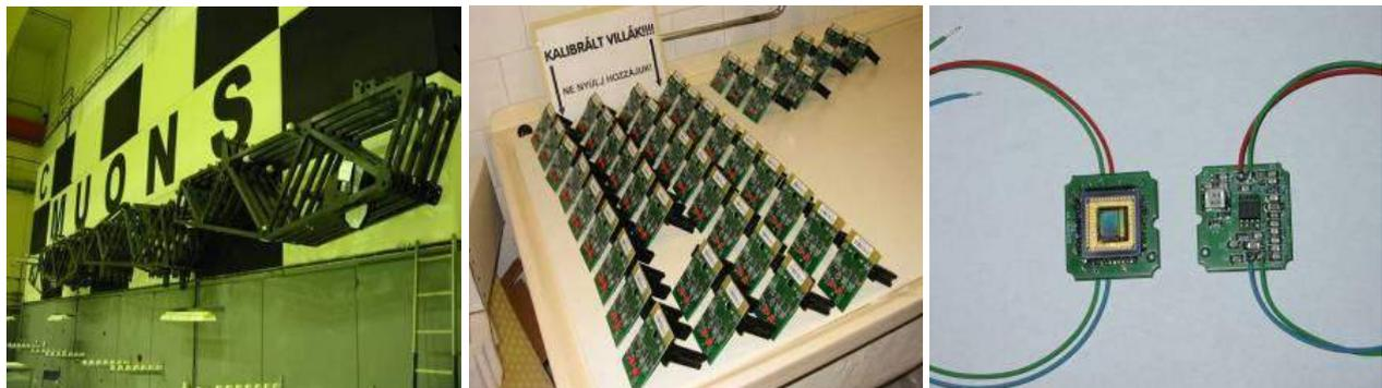
**Figure 21:** Components of the CMS position alignment system: MABs, LEDs, and video sensor left to right.
