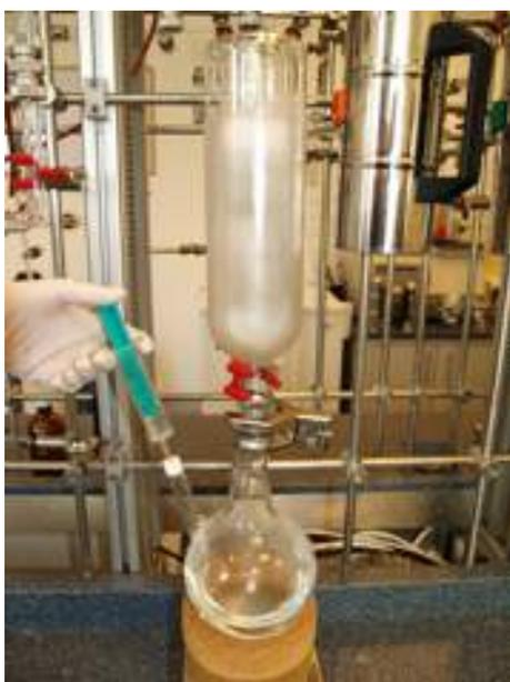
**Figure 1.** LDC water preparation setup, adapted from the University of Arizona design.
