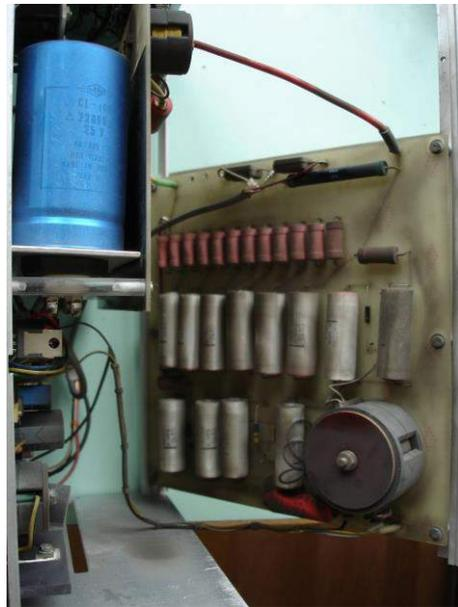
**Figure 3:** CAMAC 8kV power supply after 15 years of continuous operation at  $^{14}\text{C}$  dating laboratory.
